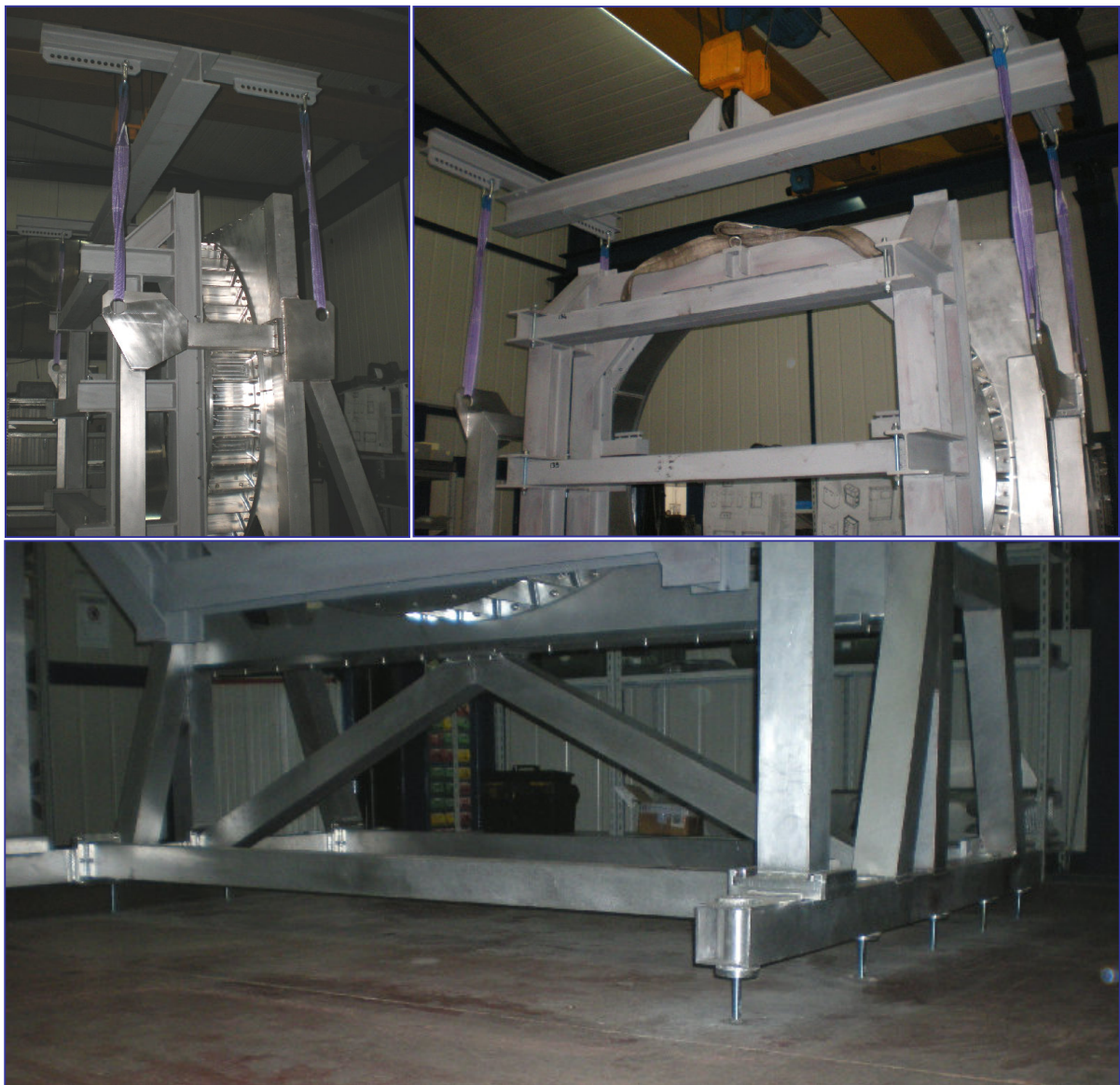
Fig. 4: Pictures of the weight load tests of the assembly
