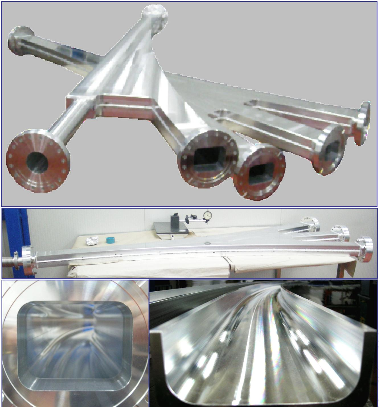
**Fig. 8: Beam extraction chambers (2-way and 3-way), and bending magnet chambers**
