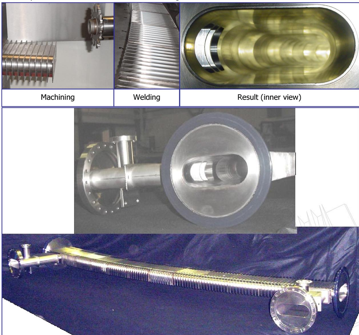
**Fig. 7: Dipole thin chambers for the Storage Ring**
