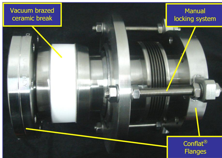
**Fig. 4: UHV bellows assembly with ceramic break**
