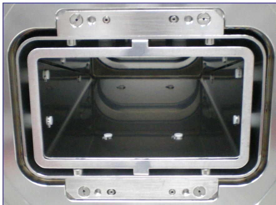
**Fig. 6: Electrodes and ceramic insulators of the pick-up chamber**
