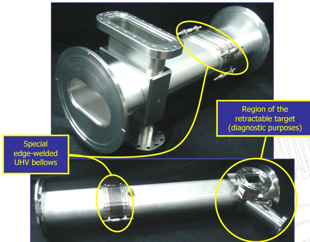
**Fig. 2: Chambers for the straight sections**
