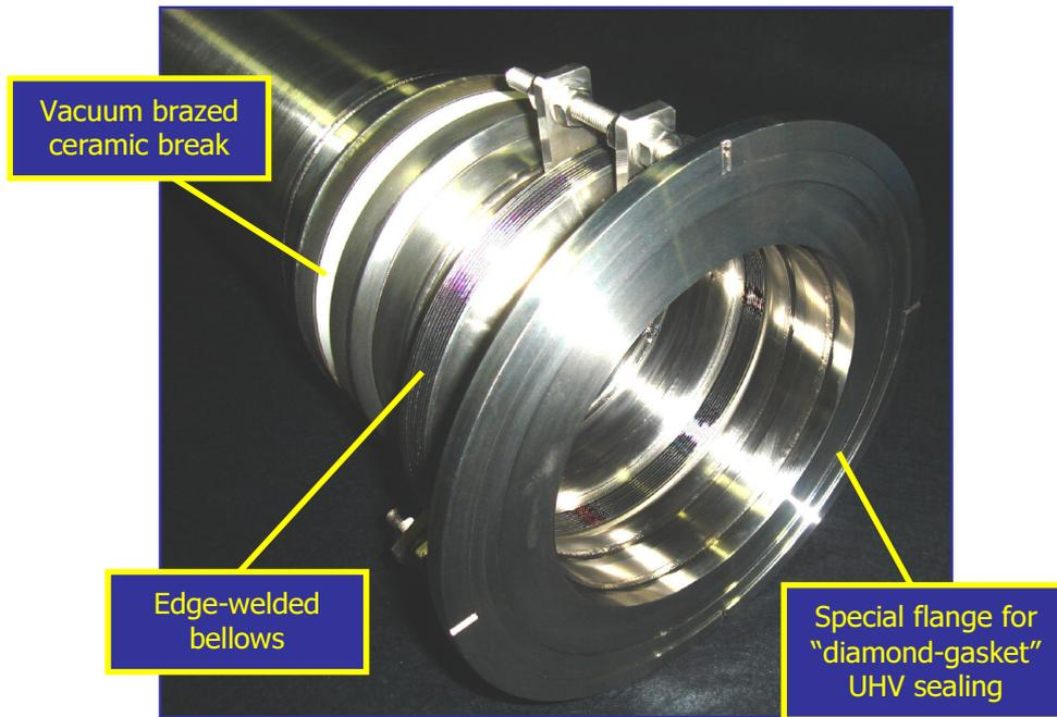
**Fig. 3: UHV chamber with edge-welded bellows and ceramic break**
