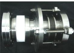
Another special application is represented by the bellows assemblies in which a ceramic break is included. This is in particular important when the electrical or thermal insulation between inlet and outlet flanges is needed. This solution requires a special vacuum brazing process and a high care and experience in the final assembling operations.
