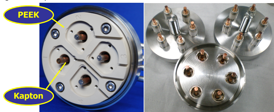
Fig. 4: TIG welding of the conductor elements to the warm flange
