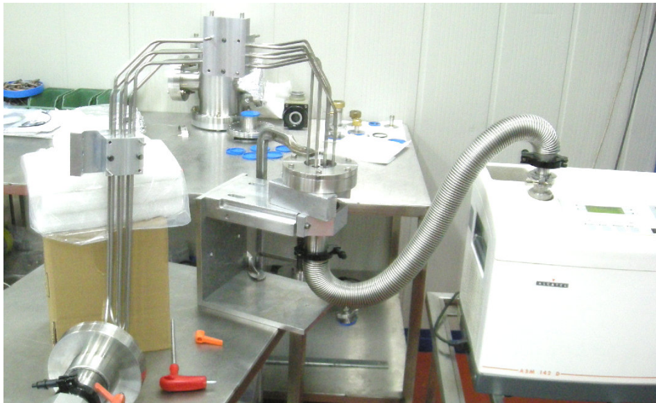
Fig. 7: Leak test of the conduction-cooled current leads
