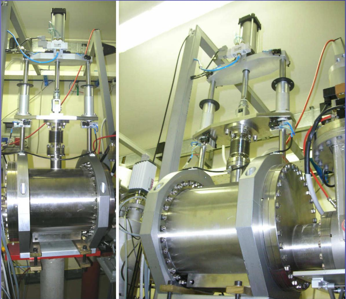
**Fig. 16: Photon shutter for the X-ray beamline at DAΦNE (LNF-INFN)**
