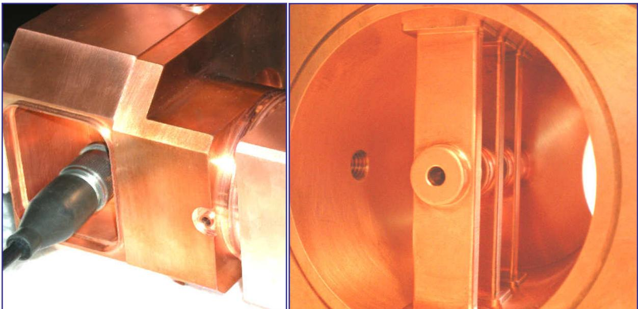
**Fig. 3: RF-cavities (S-band linear accelerator components)**
