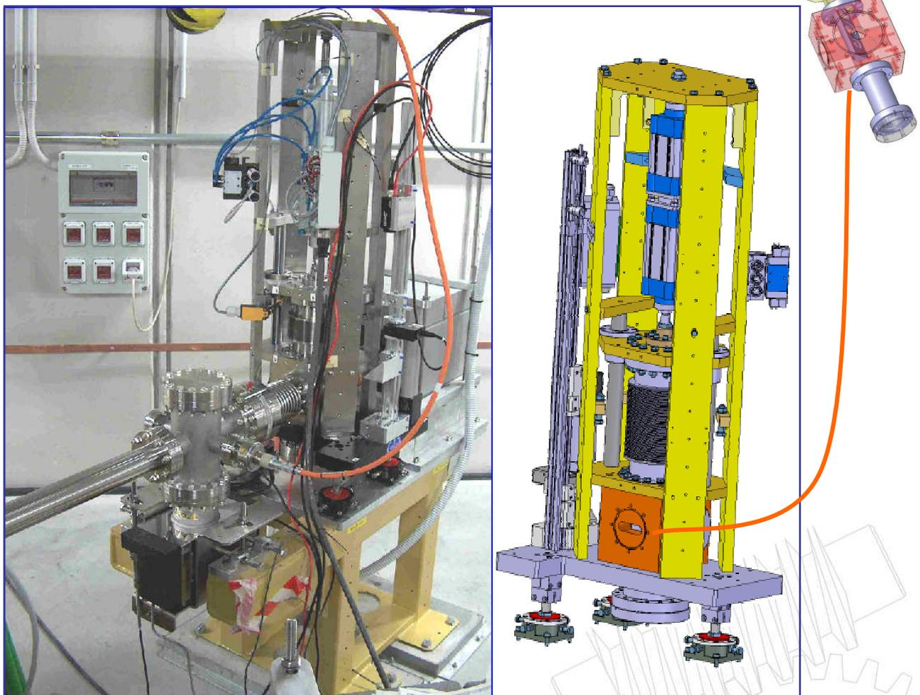
**Fig. 17: Multi-screen Wide Section for "Sincrotrone di Trieste - ITALY"**
