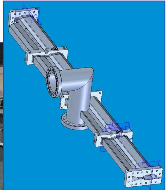
**Fig. 6: Straight UHV chamber for the ALBA Storage Ring**
