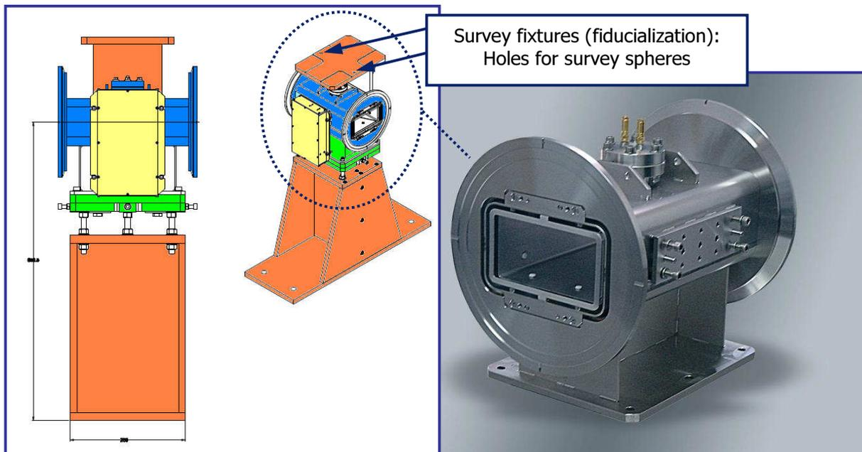
**Fig. 9: Pick-up for CNAO**
