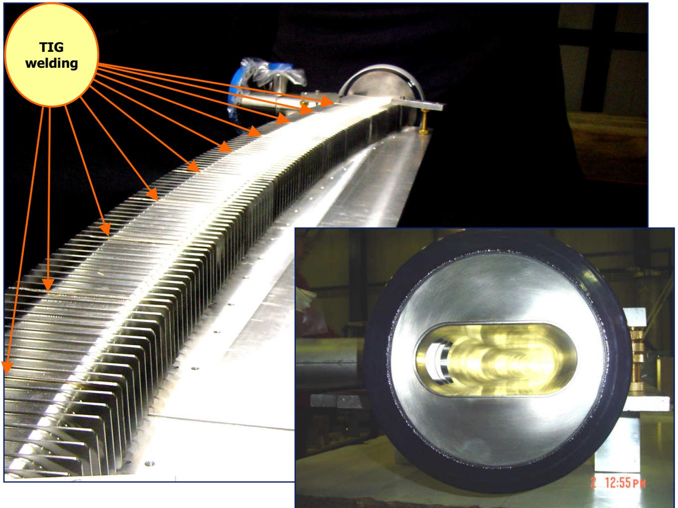
**Fig. 8: Assembled vacuum chamber for CNAO dipole**
