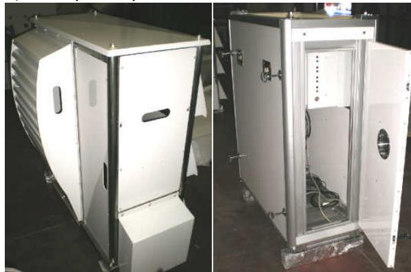
**Fig. 21: ALMA protective enclosures for cryogenic units**
