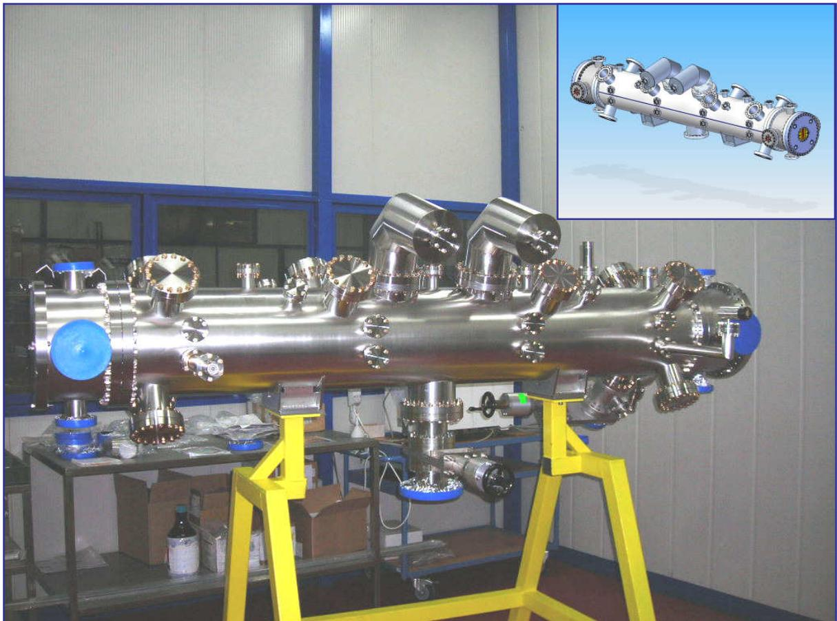
**Fig. 7: Insertion device for Diamond Light Source**
