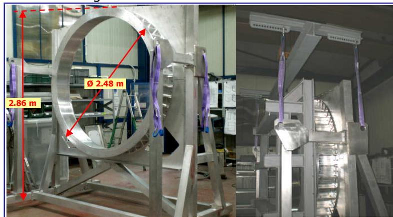
**Fig. 20: ESO Integration and Handling Stand Structure**
