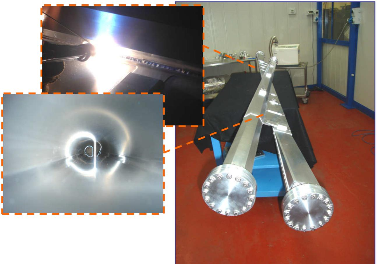
**Fig. 10: Vacuum chamber for the beam-crossing region of DAΦNE**
