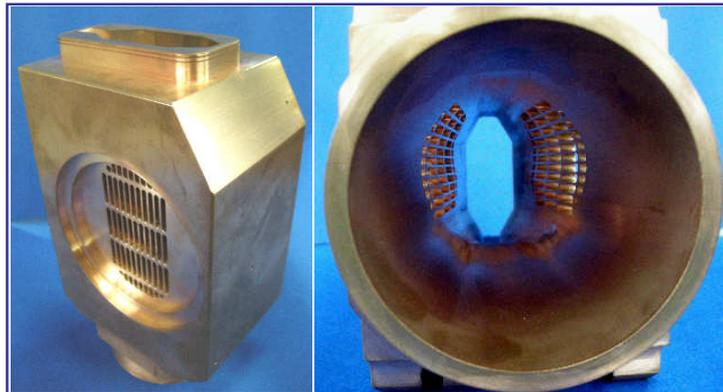
**Fig. 14: OFHC Copper absorber completely machined**
