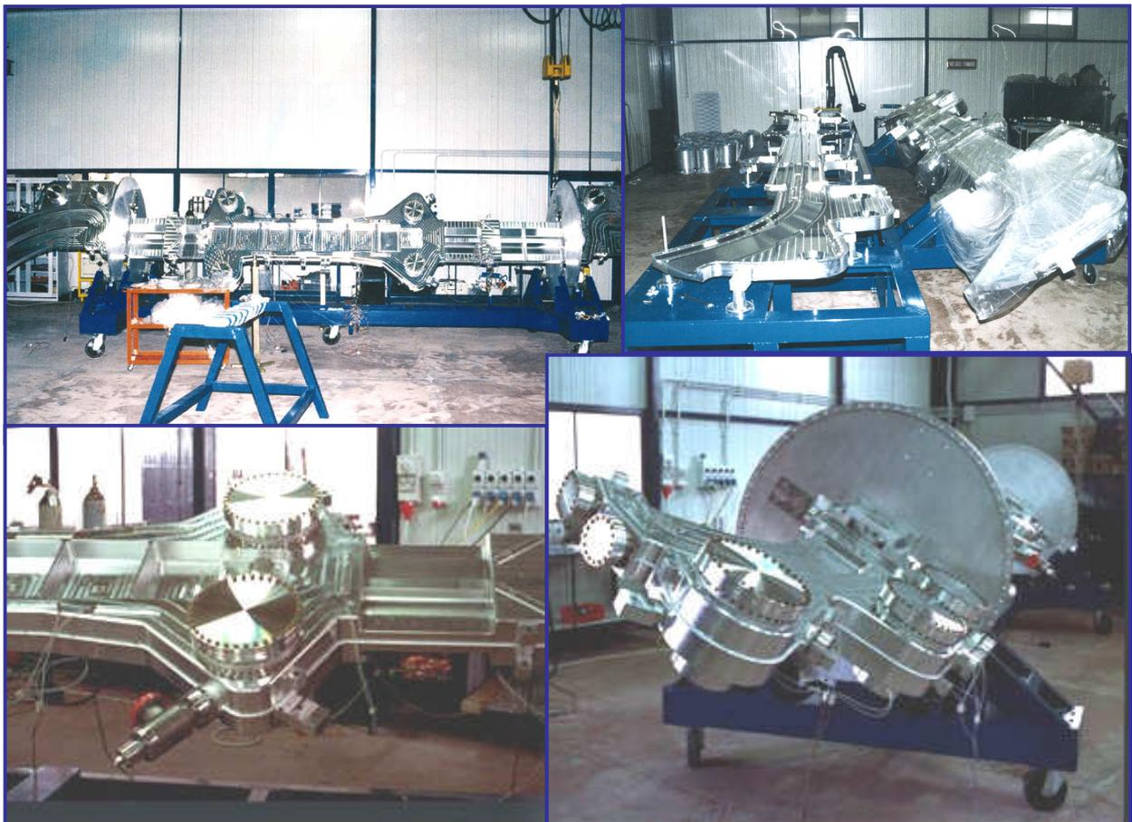
**Fig. 11: Manufacturing process for chambers of the DAΦNE bending magnet**
